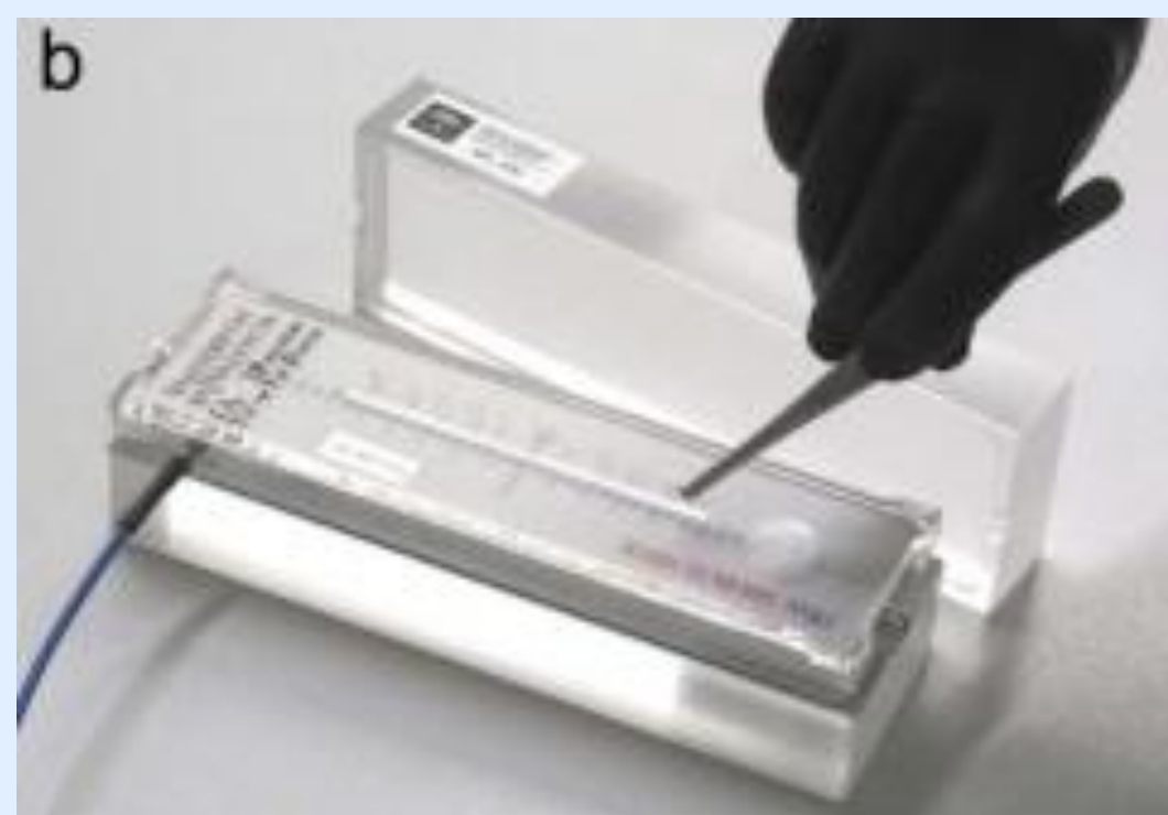
Figure 1: PTW SourceCheck flat chamber. Source: Tornero-Lopez (2015)
